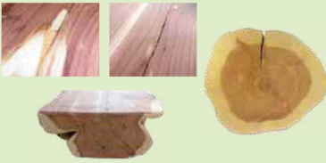
Natural Cracking and Checking
