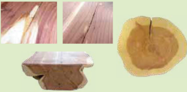
Natural Cracking and Checking
