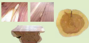
Natural Cracking and Checking
