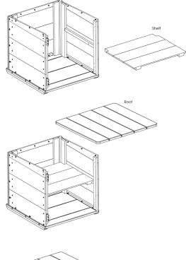
Slip the Roof into place. Secure the Side Panels and Back Panel to the Roof, using nine screws.
