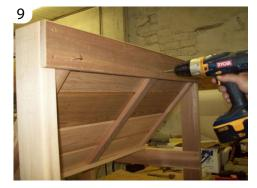
Attach the triangular piece to the bottom of the base using  $1 \frac{1}{2}$ " screws. Repeat on other side.
