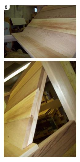
Attach the top of the bin panel to the outside frame using 1 <sup>1</sup>/<sub>2</sub>" screws. Repeat for other side.
