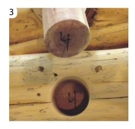
Next, line up each leg with the mark found on the bench to ensure the leg is turned the proper way.
