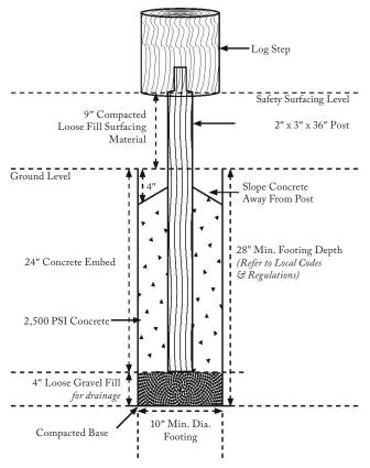
After all of the footing holes have been prepared, place the posts into their respective holes. Make sure each log step is level and plumb in the footings. Use scrap wood to brace into position if necessary.
