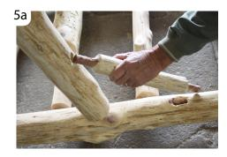
After dry-fitting the pieces, disassemble. Apply a line of Exterior Grade Construction Adhesive halfway in each hole along the sides of each hole. Repeat **steps 2-5**.
